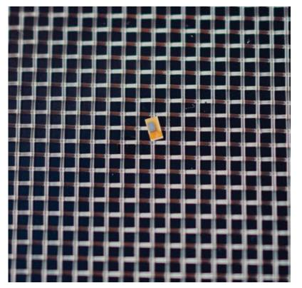
A fabricated Vertical Cavity Surface Emitting Laser (VCSEL) device that are difficult to implement, including very high accuracy of their light emission color, shape, and polarization, as well as the ability to operate at extremely high temperatures. The Technion successfully developed such VCSELs, that even outperform the best commercially available competitors.
